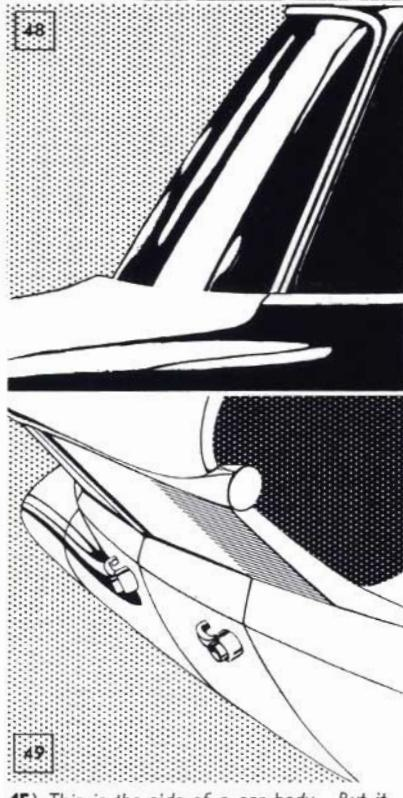
**45)** This is the side of a car body. But it is no ordinary one. It is the side of a Citroen ID or DS. Its curve has been carefully designed to offer the least resistance to cross-winds and to place the aerodynamic center of pressure to the rear of the center of gravity in order to increase the aerodynamic stability of the vehicle.
